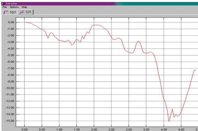
Figure 2. 16" Blue cable female Z-Trace to male VP to female Z-Trace with cable and Z-Trace connectors de-embedded (-3 dB at 1.2 GHz)
