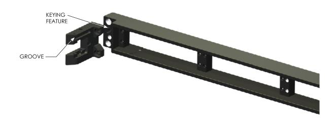
The rotation blocks were also designed with a tongue and groove feature to prevent placing the ITA in upside down.
