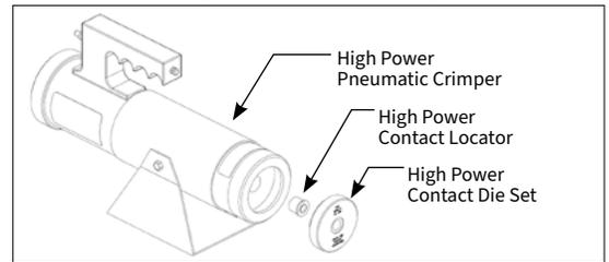
Figure B. Exploded view of pneumatic crimper.
