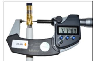
Figure D. Measuring crimp.
