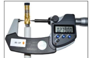
Figure D. Measuring crimp.
