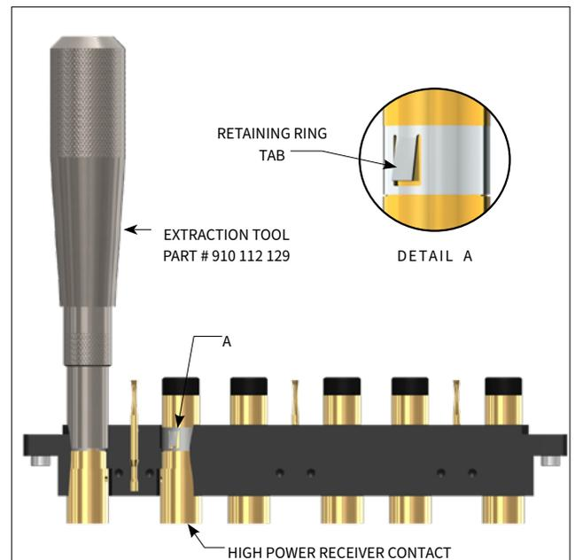
Figure B. Fully seat extraction tool before depressing.
