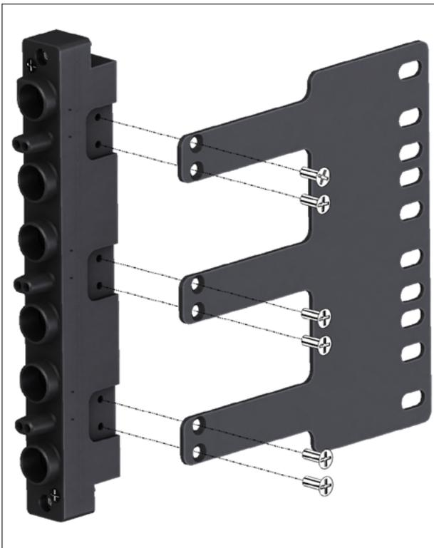
Figure A. 90 Series Strain Relief Installation.
