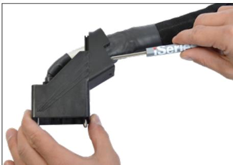
Figure C. Attach cable clamp housing.
