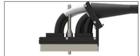
Figure E. Applied shrink tube.
