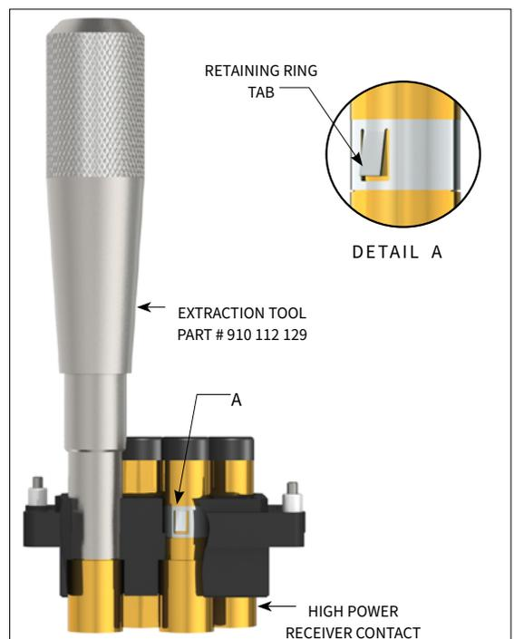
Figure C. Fully seat extraction tool before depressing.
