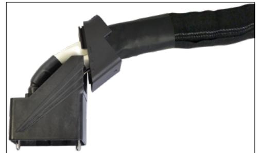
Figure B. Apply sleeving and shrink tubing.
