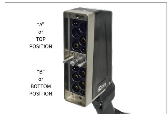
Figure B. Correctly loaded ITA contacts in iCon.
