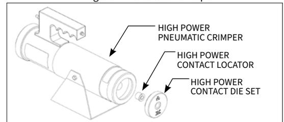
Figure B. Exploded view of pneumatic crimper.
