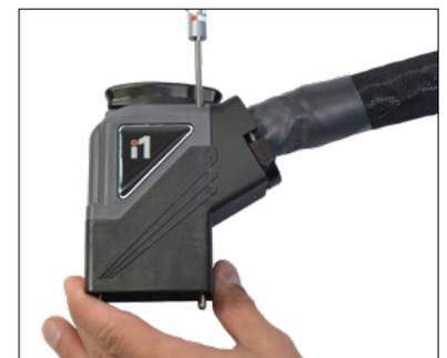
Figure E. Attach engagement housing.
