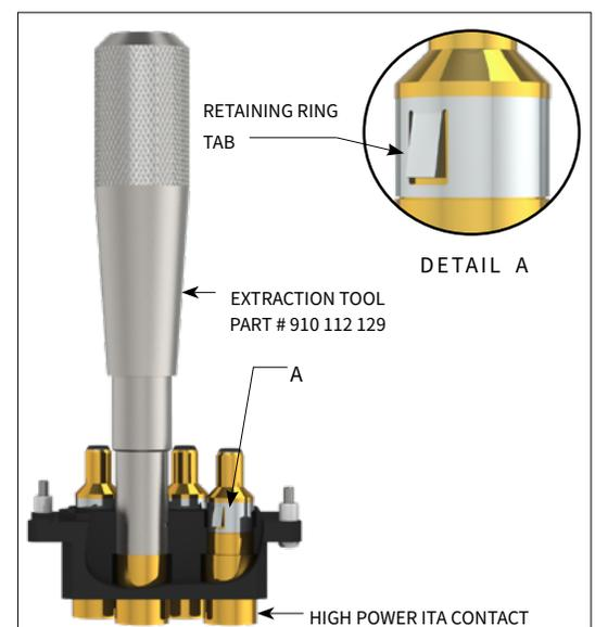
Figure B. Fully seat extraction tool before depressing.
