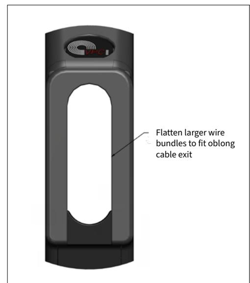
Figure B. Cable clamp exit area.
