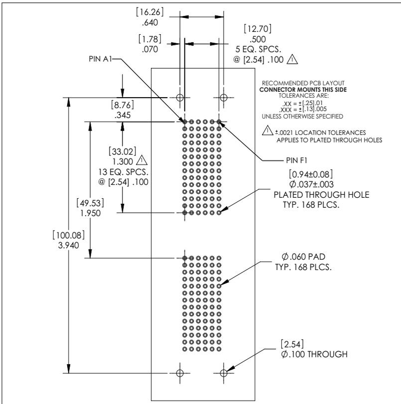
**(Figure A)** PCB layout for i2 receiver, Part # 310 130 101. Through hole and pad diameters are for VPC QuadraPaddle male Adapter Contact, Part # 610 138 117. The size of these holes may be different if a header from a different manufacturer is used. Connector mounts this side.
