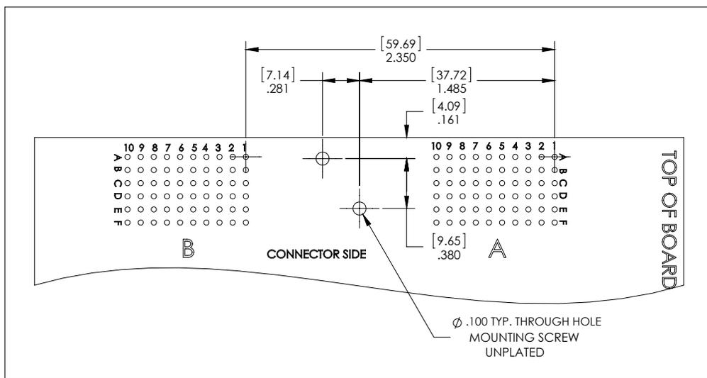
(Figure B) Two header layout for 310 130 104 receiver.
