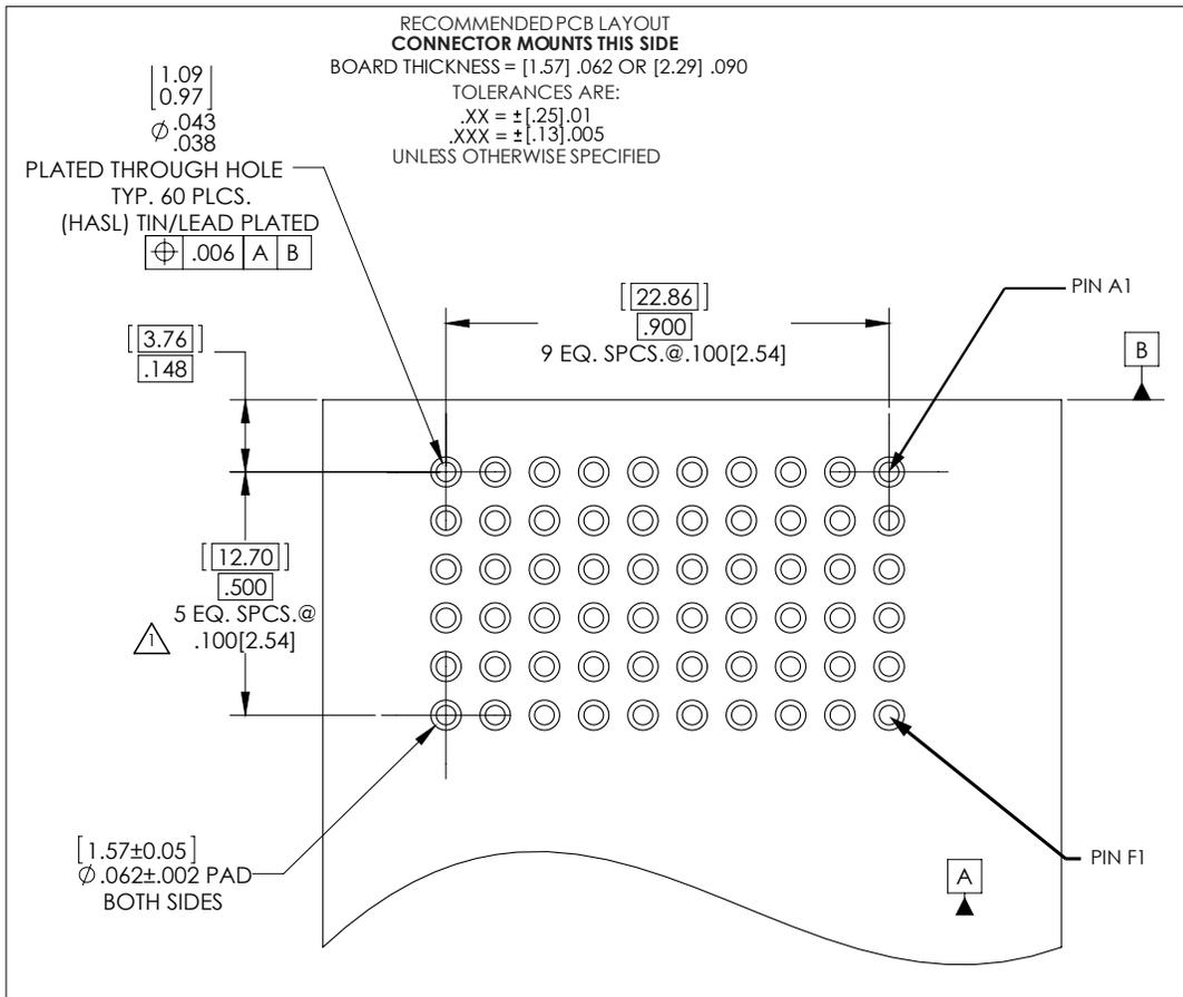
(Figure A) PCB layout. Connector mounts this side.
