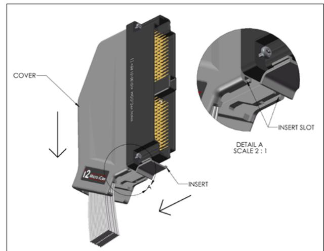
Figure C. Slide cover down and install insert.
