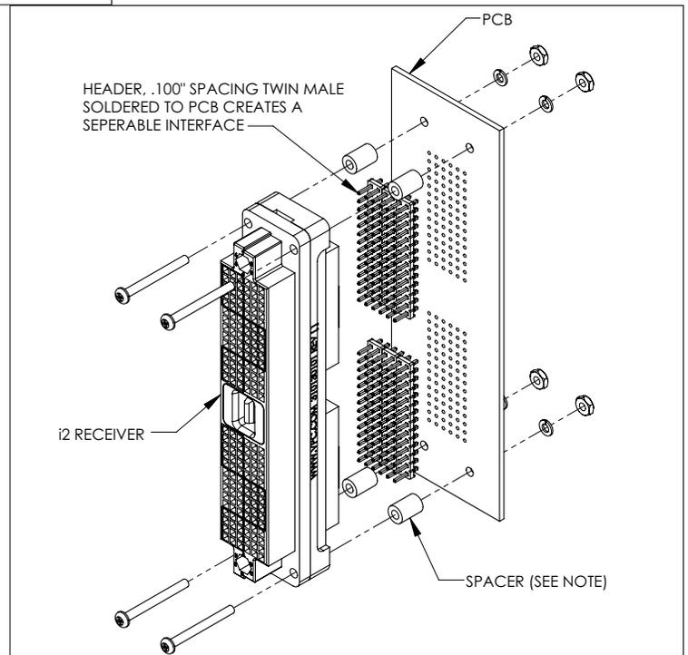
**(Figure D)** A PCB can be mounted directly to the back of an i2 receiver as shown above. Four 2-56 or M2 screws are required to mount the receiver. Spacers may be needed to prevent unwanted stress on the PCB.
