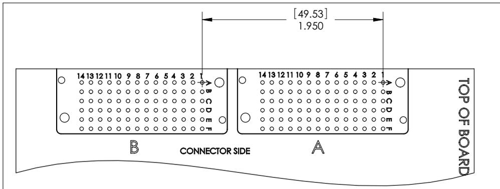
**(Figure B.)** Two header layout for 310 130 101 receiver.
