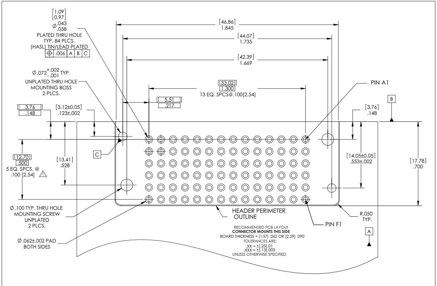
**(Figure A.)** PCB layout. Connector mounts this side.
