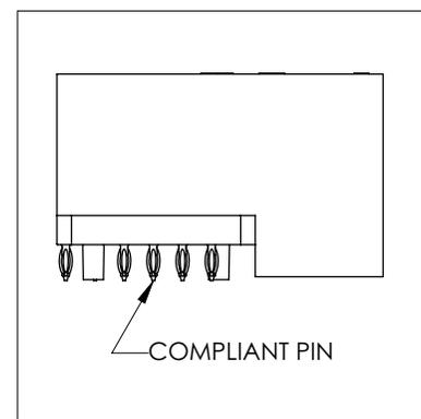
(Figure C) Compliant header pin.
