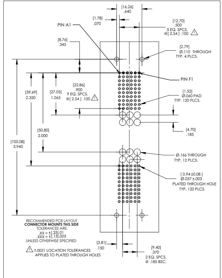
**(Figure B)** PCB layout for i2 hybrid receiver, Part # 310 130 104. Through hole and pad diameters are for VPC QuadraPaddle male Adapter Contact, Part # 610 138 117. The size of these holes may be different if a header from a different manufacturer is used. Connector mounts this side.
